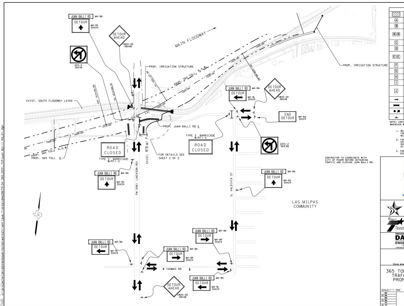
LEGEND CONSTRUCTION PHASE WORK ZONE PVMT MARK (NON-REM) 4" WHITE SOLID WORK ZONE PYMT MARK (NON-REM) 4" YELLOW SOLID WORK ZONE PYMT MARK (NON-REM)
